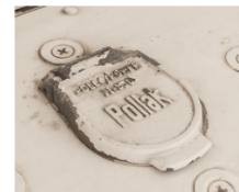
External Power Receptacle
